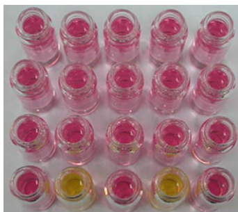
Figure 3. The color change of 2 (5.6 \mu\text{M} ) in DMF–H 2 O 9:1 (v/v) in the presence of 20 equiv of certain amino acids. From left to right and top to bottom: absence of amino acid, phenylalanine, threonine, arginine, histidine, asparagine, leucine, alanine, proline, valine, glycine, lysine, glutamine, methionine, isoleucine, serine, cysteine, tryptophan, homocysteine, and aspartic acid.
